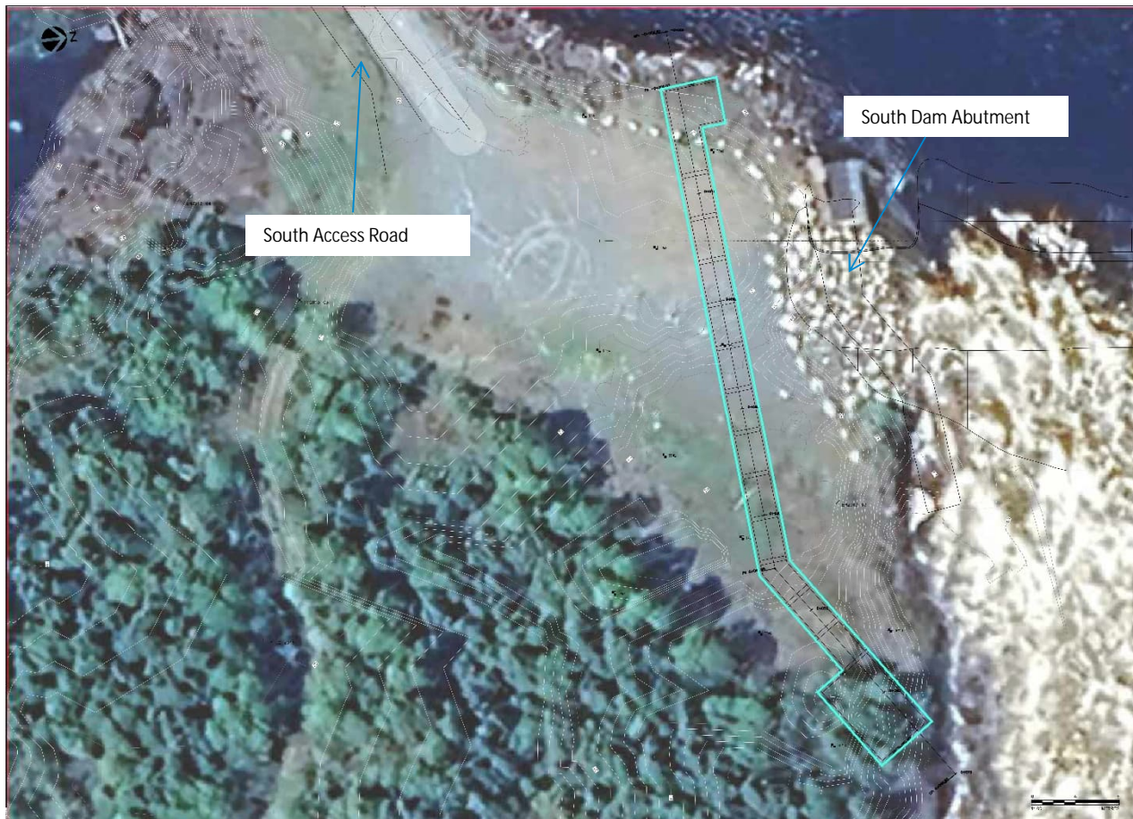
Figure 2-6 Layout of the New South Side Fishway
