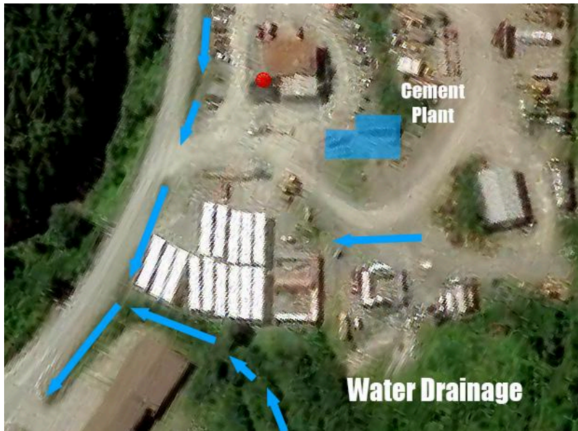
Figure 4. Proposed Concrete Batch Plant Water drainage
