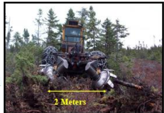
Normal Trench Spacing
