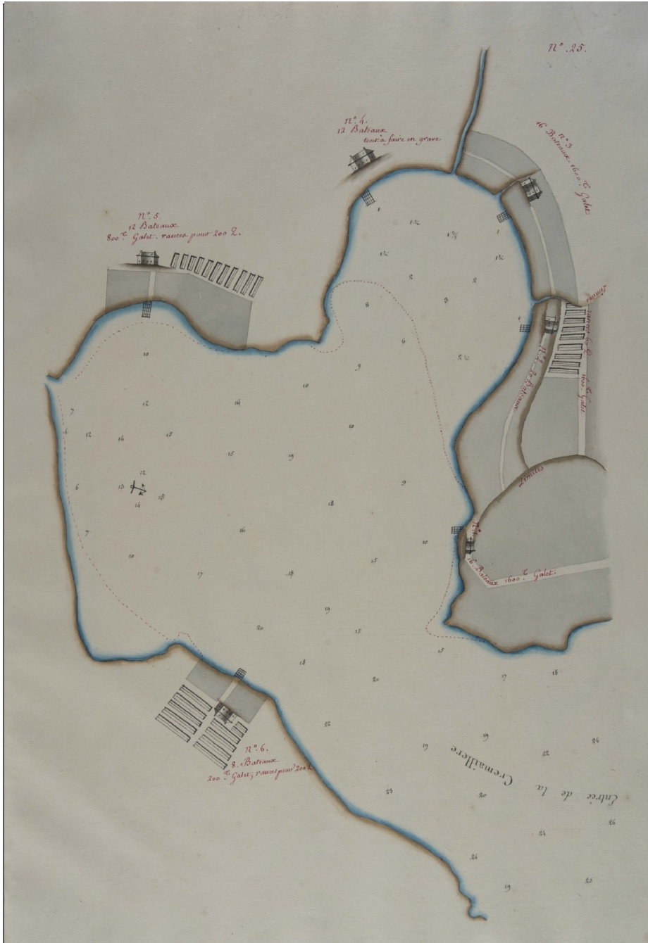
A chart of Crémaillière harbour, Letourneur [1784]. The Banc à l'Ours fishing room and Batteau Cove are at bottom, left, with a structure backed by ten rances 4 and fronted by two galets, judged sufficient for eight boats. The other five fishing rooms in the harbour are judged 12-20 boats' room, for a total capacity of 84 boats.
