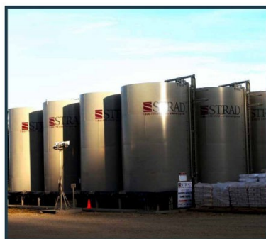
Figure 4-7 Typical Liquid Mud Tank Farm Arrangement
