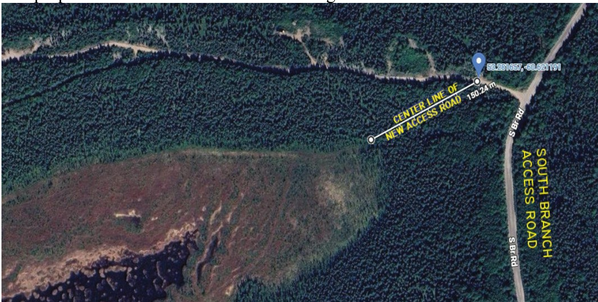
Figure 2 – Center Line of Proposed New Access Road
