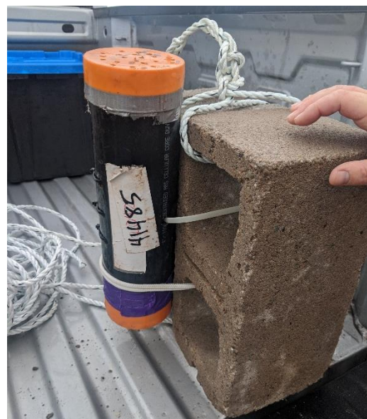
Figure 2.3: RBR Pressure Gauge Anchor Setup.
