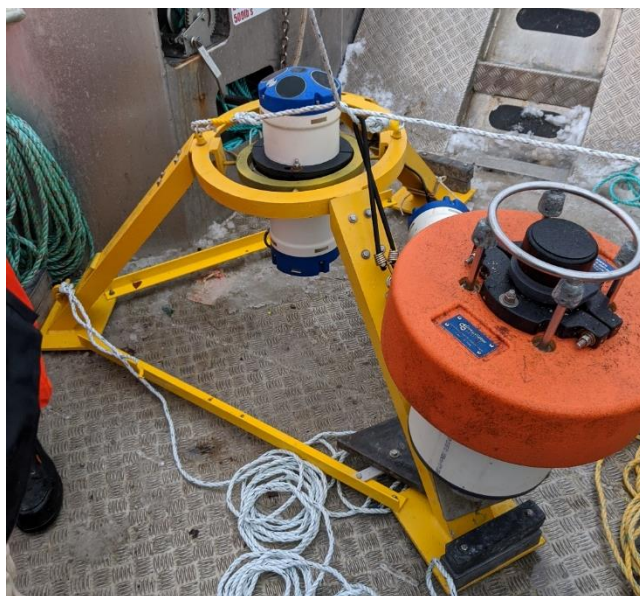
Figure 2.2: ADCP Deployment Setup.
