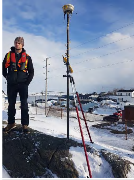
Figure 3.3.3 – Trimble rover setup over 82G2332.
