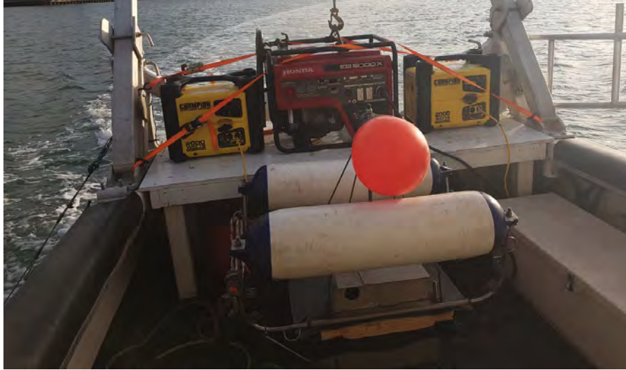
Figure 3.1.4 – Boomer system on deck after retrieval.
