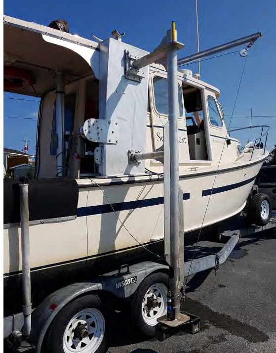
Figure 3.3 – Multibeam transducer on SeaQuest over-the-side mount.
