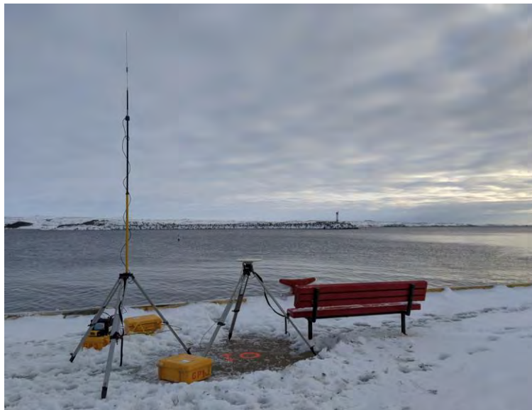
Figure 3.1.1 – Trimble RTK-GPS base station set up on CSR1945 BS1f.
