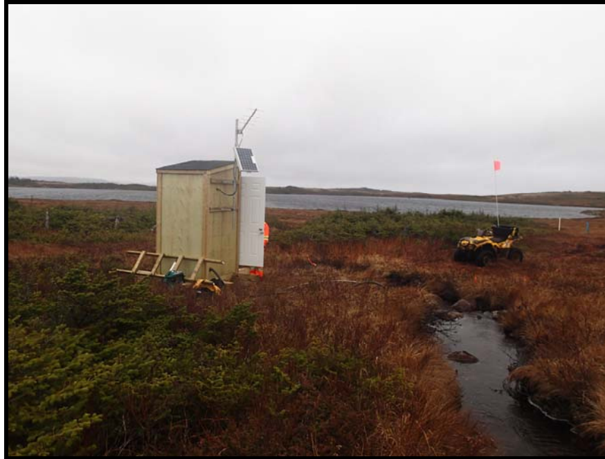
Figure 2: Real-Time Water Quality and Quantity Station at Outflow of Grebes Nest Pond.
