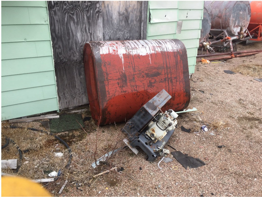
Photo 9 – Camp / Antenna Areas and AES Compound: Full 900L AST lying against south-facing exterior wall of Camp Garage Building (emptied and removed as part of the current assessment). Looking north.
