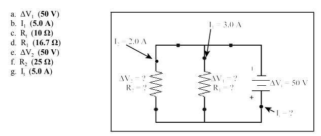
16. In the circuit shown,  $R_1 = 20 \Omega$ . The potential drop across  $R_1$  is 10 V; across  $R_2$ , it is 20 V. Determine the following:
