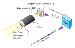
It is at this point the cameras vary in how the information (images and sound) is stored. Digital video records the signal as a series of 0's and 1's in digital format.
