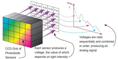
Analog video is captured using a lens which is focused on a CCD. The CCD has an array of 300 000 to 500 000 photodiode light sensors (photosites). Each sensor corresponds roughly to a pixel. The photodiodes respond to light colour and intensity. As light falls on a point, there is a corresponding voltage produced.
