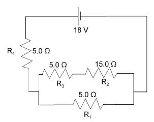
The 5.0  $\Omega$  and 15.0  $\Omega$  resistors are in series, so the resistance in that series branch is 20.0 Ω. Then the parallel branch has a total resistance given by:
