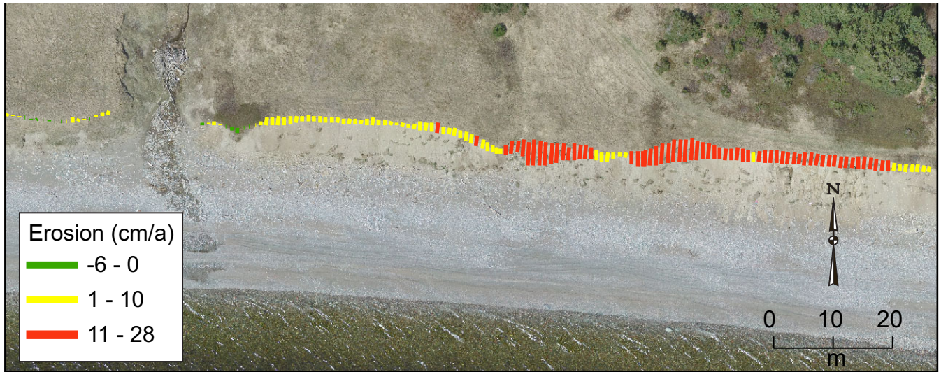
Figure 10. The DSAS analysis of coastal erosion from 2000 to 2016 along Seaside Drive, Kippens. Only the coastline west of Williams Lane (Figure 8) is displayed, to allow the coloured bars to be visible. Colour and bar length represent the spatial variation in erosion. The length of the bars represents the total amount (measured in cm) of cliff-top erosion for the period of analysis; the longer the bar length, the greater the amount of coastal erosion. Red, yellow and green bars denote accelerated, moderate and minor erosion respectively.
