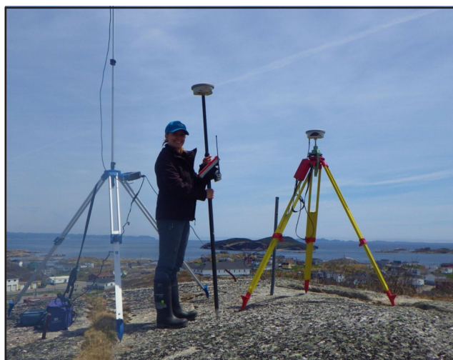
Plate 9. Real Time Kinematics survey equipment. The base station (yellow tripod) is set up over a previously established survey monument with known coordinates. The base station transmits reference position information to the roving receivers through the radio (blue tripod). The hand-held roving receiver, consisting of an antenna and field controller attached to a telescopic pole, is used during surveying.
