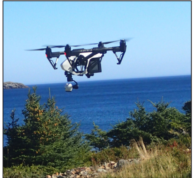
Plate 11. The DJI Inspire 1 Quadcopter is a light UAV equipped with a digital camera, and is controlled by an operator on the ground using a hand-held controller.
