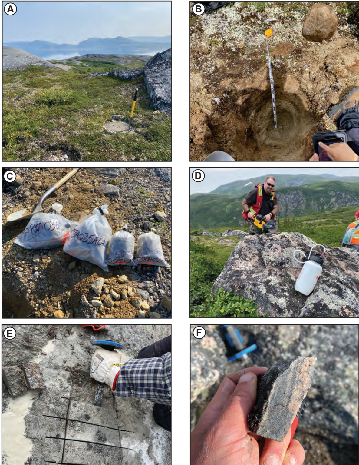
Plate 2. A) Example of frost boil targeted for till sampling at site 25RBA065; B) Test-pit dug to expose the C horizon for sampling at site 25RBA023; C) Showing sample bags and size for different analysis, the larger for indicator-mineral identification and the smaller for geochemistry and a duplicate sample to assess QA/QC at site 25RBA035; D–F) Examples of how samples are collected for cosmogenic exposure age dating from site 25RBA057 where (D) the erratics are scored in a grid pattern to allow (E) chiseling out of the required sample (F) for exposure age dating.
