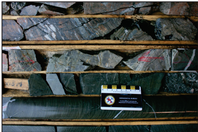
Plate 2. Basal contact of flow-banded rhyolite with underlying thinly-bedded green siltstone at the Big Easy prospect. Note the weakly developed, locally crustiform-banded, centimetre-scale quartz veins crosscutting the rhyolite unit. This veining, developed along the margin of the rhyolite, is associated with anomalous gold (69 ppb) and molybdenum (18.5 ppm) over 1 m (Delazzer and Dimmell, 2012; DDH BE-11-05; 217 m depth).
