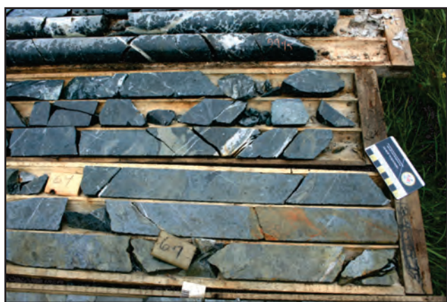
Plate 40. Gradational transition from an Fe–Mg chlorite altered intermediate volcanic rock and related hyaloclastite to muscovite and then paragonite white mica alteration. Photograph is taken just above the mineralized zone shown in Figure 31; DDH MM-19-033, 64 m depth.
