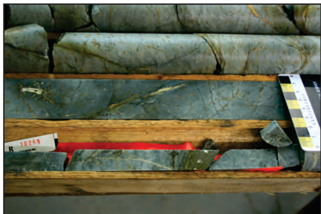
Plate 36. Silicified felsic volcanic rock, locally crosscut by cm-scale sulphide veining. Sample from the bottom of the photograph returned 0.6% Cu, >1.0% Pb, >1.0% Zn, 98 g/t Ag and 0.72 g/t Au over 0.03 m (Thurlow et al., 1987); DDH BJ-083, 107 m depth.
