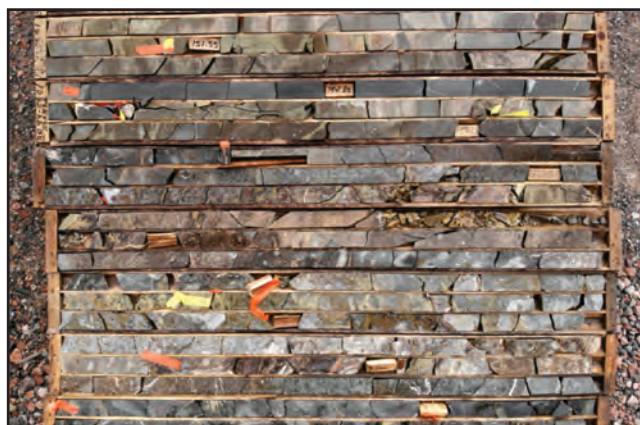
Plate 28. Transitional zone from phengite-dominated (top) into muscovite-dominated white mica spectral signatures developed near the sharp contact between a polymict lithic breccia and overlying weakly feldspar-phyric intermediate volcanic rock; DDH BR-99-08-001, 144–180 m depth. Note that one row of drillcore is approximately 1.5 m in length.
