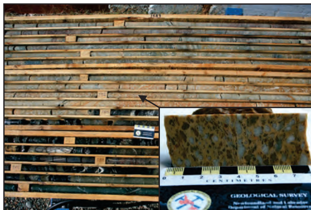
Plate 10. Quartz-phyric rhyolite characterized by muscovitic illite and paragonitic illite spectral signatures, interbedded with relatively unaltered mafic volcanic rocks characterized by Fe-Mg-chlorite; Sandfill prospect, DDH H-1683, 156–180 m depth.
