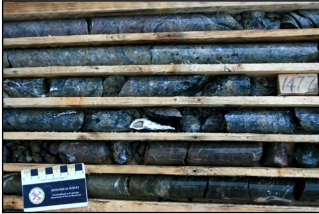
Plate 11. Quartz-phyric rhyolite characterized by muscovitic illite spectral signature overlying relatively unaltered mafic volcanic rocks characterized by Fe-Mg-chlorite (bottom of photo); Sandfill prospect, DDH H-1910, 450 m depth.
