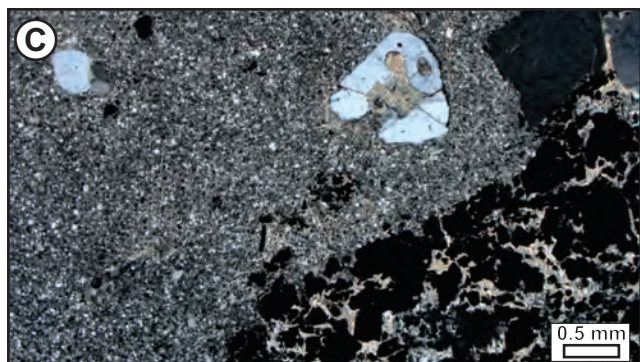
Plate 17. A) Paragonite-dominated white mica alteration crosscut by pyrite-rich sulphide veining. Note the veins are hosted by a strongly altered, quartz-phyric, felsic volcanic rock; B) Plane-polarized light photomicrograph of sample shown in (A). Note the locally developed resorption texture in the quartz phenocrysts of the host rock; C) Cross-polar photomicrograph of (B) highlighting the intense white mica alteration of the host rock; D) Reflected light image of (C) showing the pyrite (Py)-dominated sulphide vein. Note that the pyrite is host to fine-grained inclusions of galena based on SEM imaging.
