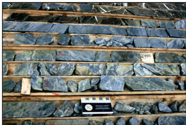
Plate 12. Paragonitic illite–montmorillonite altered felsic volcanic of the Powerhouse prospect; DDH BE-97-020, 30 m.
