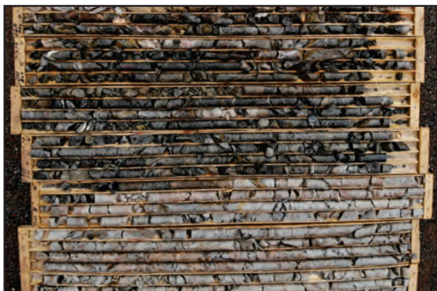
Plate 15. Sharp transition, from Fe–Mg-chlorite–muscovitic illite dominated alteration to intermixed paragonite–paragonitic illite–montmorillonite and Fe–Mg-chlorite–paragonitic illite assemblages. Powerhouse prospect, DDH H-3319, 40 to 64 m. Note that one row of drillcore is approximately 1.5 m in length.
