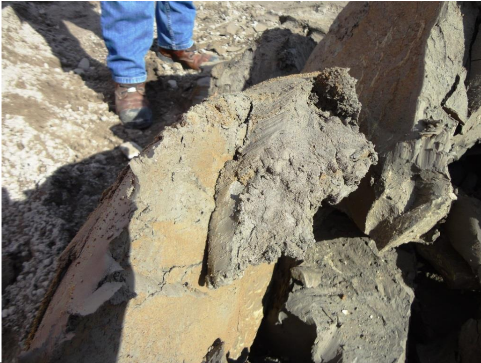
Photo 3.15: Upstream slope- Excavated greenish grey “lower clay” from the south end of the cut-off. The lower clay is a firm, plastic clay with low sensitivity. This material is at approximate el 20m along most of the upstream face and is the impervious material that the base of the cut-off wall is seated in.
