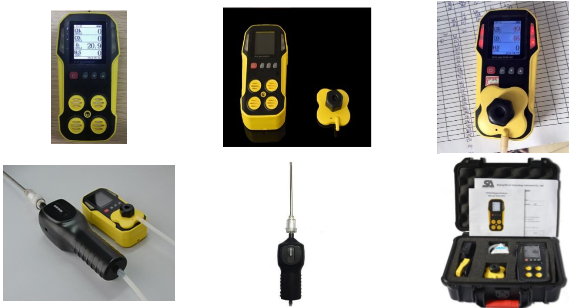
Figure 4. The portable biogas analyzer
