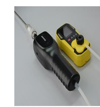
Biogas sampling pump-probe connected to the device
