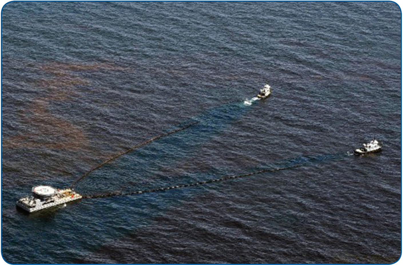
These boats are called skimmers and they help clean up oil spills.
