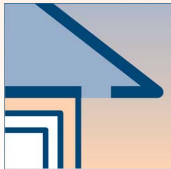
◀ Soffit vent too close to exterior wall
