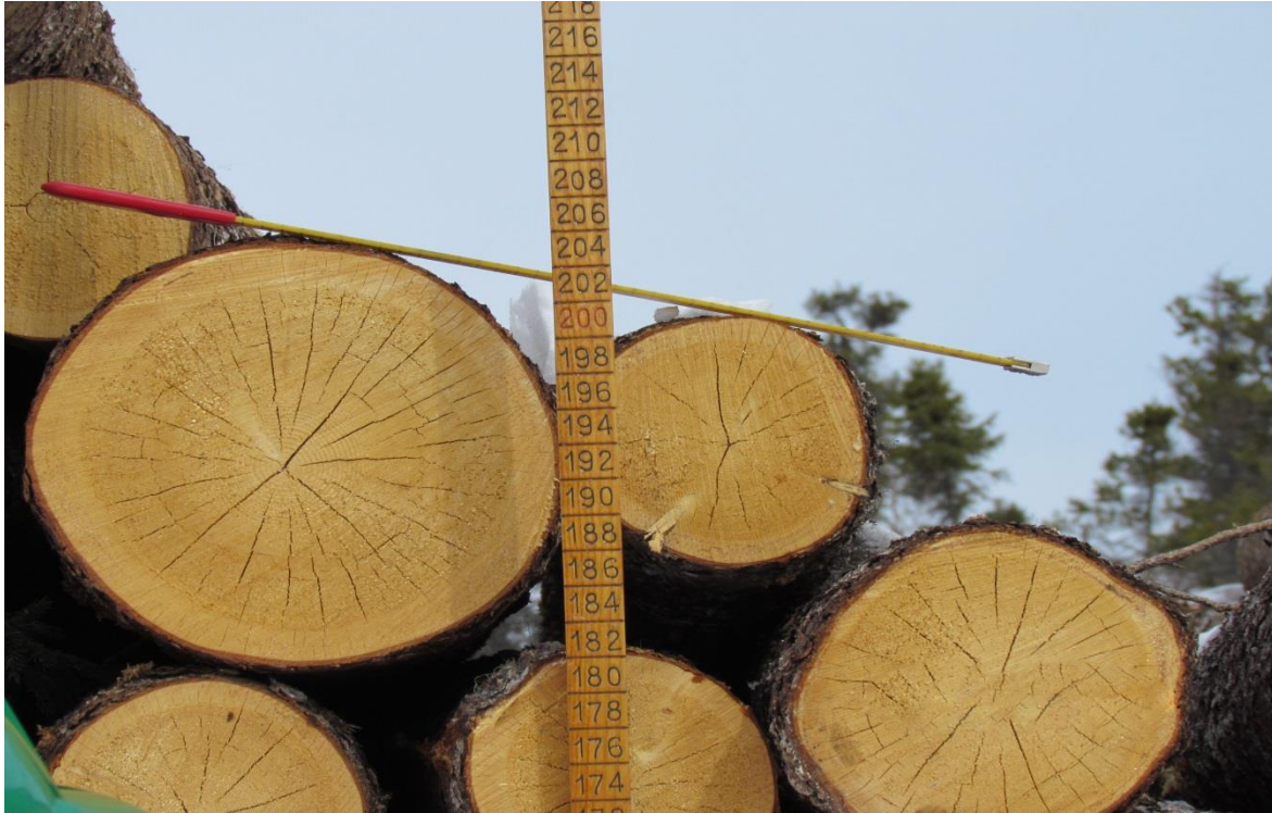
FIGURE 6 - HEIGHT READING USING EXTERIOR TANGENT METHOD, IN THIS CASE THE READING IS 202 CM
