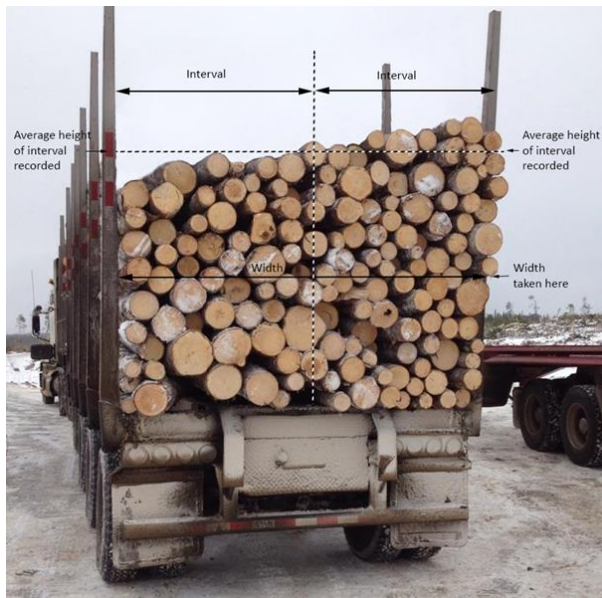
FIGURE 23 - RECORDING AVERAGE HEIGHT – WOOD STACKED SLOPING FROM ONE SIDE
