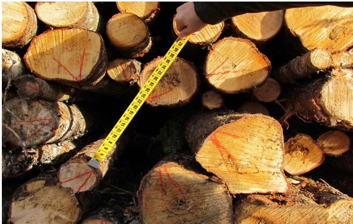
FIGURE 15 - VOID MEASUREMENT IN STACKED WOOD
