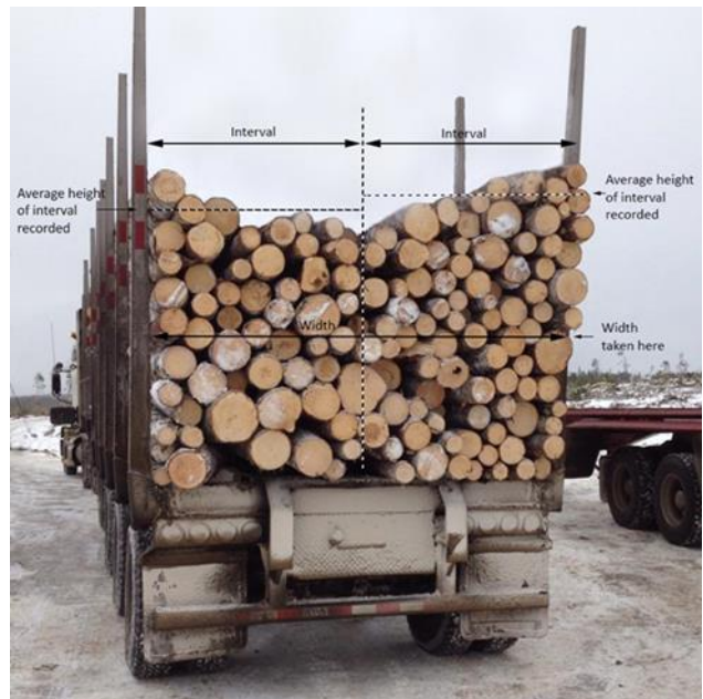
FIGURE 20 - RECORDING AVERAGE HEIGHT – WOOD STACKED SLOPING TOWARD CENTER
