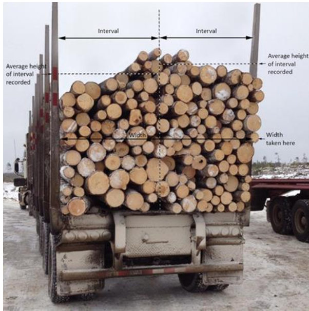
FIGURE 21 - RECORDING AVERAGE HEIGHT – WOOD STACKED SLOPING FROM CENTER
