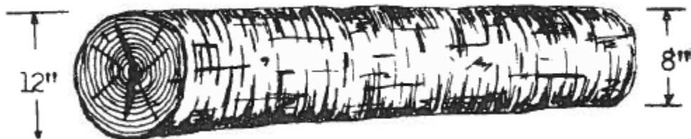
FIGURE 29 - NEWFOUNDLAND AND LABRADOR LOG RULE - LOG SHOWING HEART CHECK
