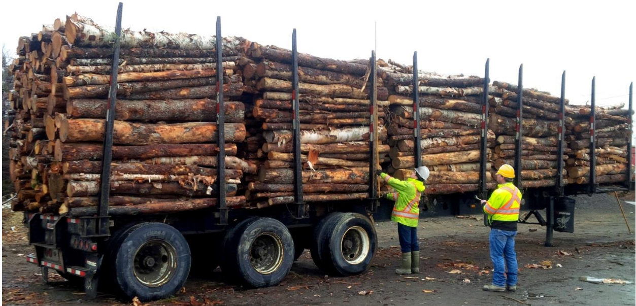
FIGURE 18 – SCALING LONGITUDINALLY STACKED WOOD ON A TRAILER
