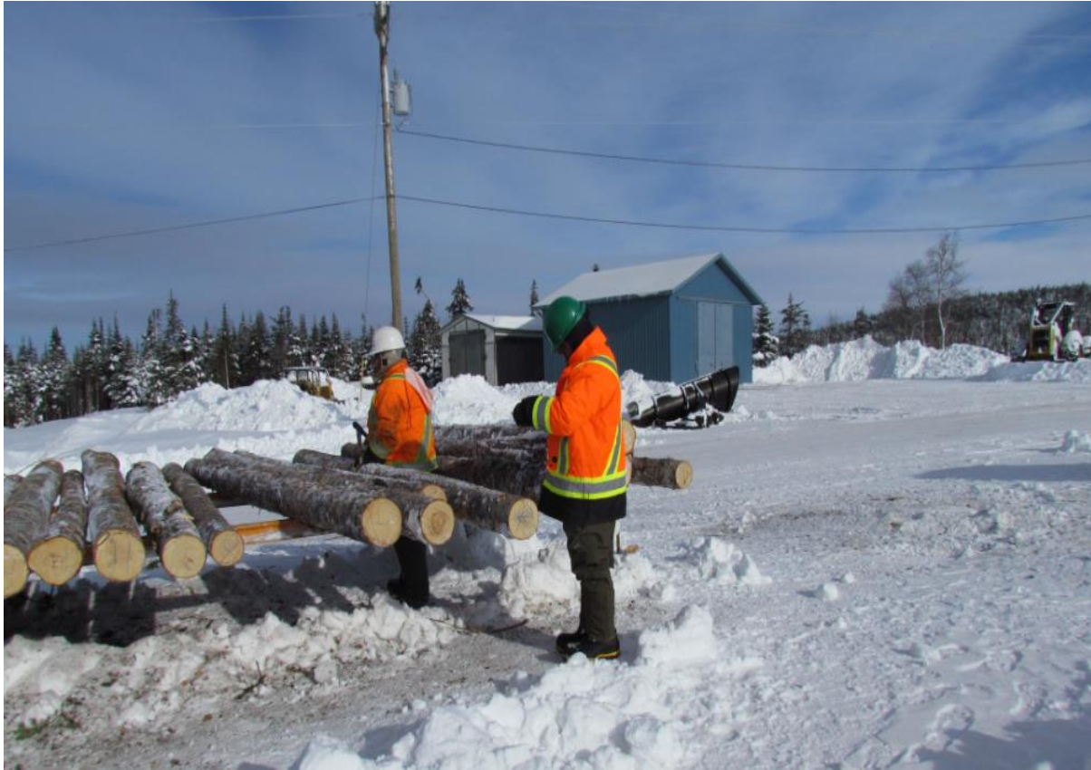
FIGURE 40 - SAWLOG SCALING (USING SMALIAN'S FORMULA)
