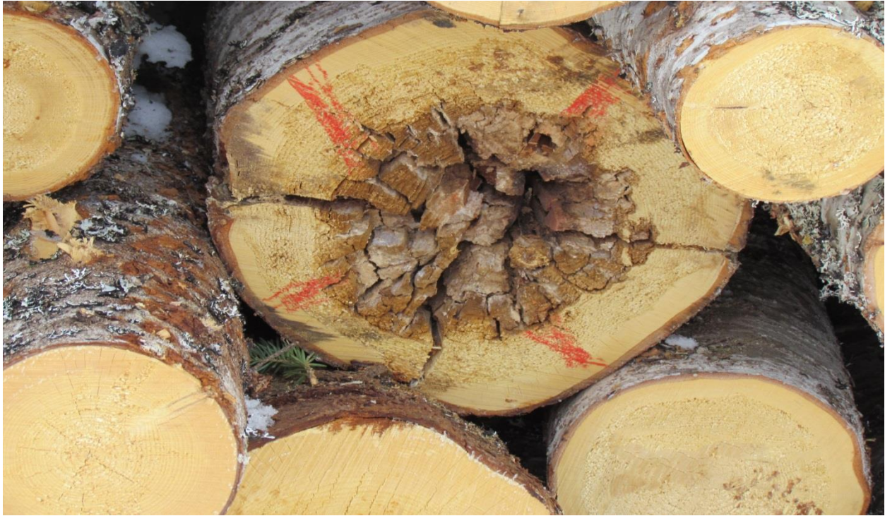
FIGURE 16 - CULL MARKING IN STACKED WOOD
