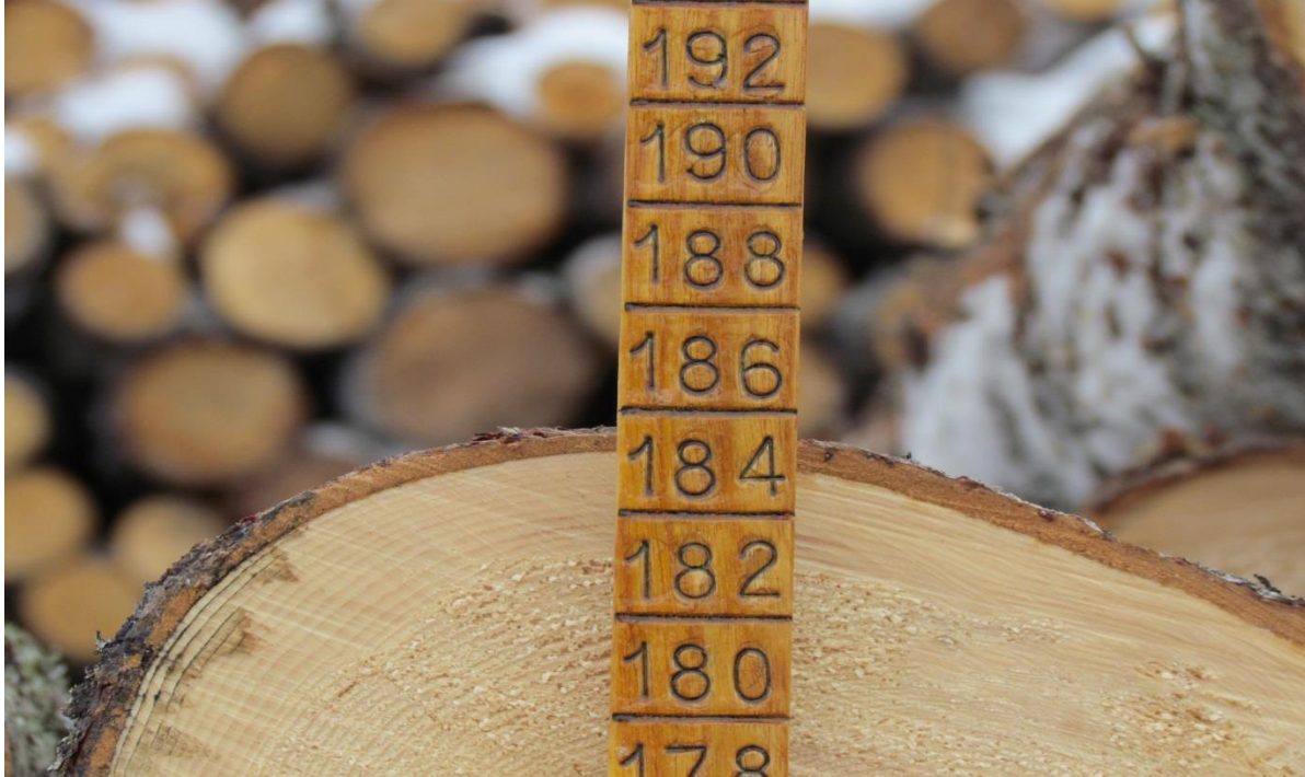
FIGURE 13 - HEIGHT READING ON A SCALE ROD – IN THIS CASE, THE HEIGHT IS 184 CM
