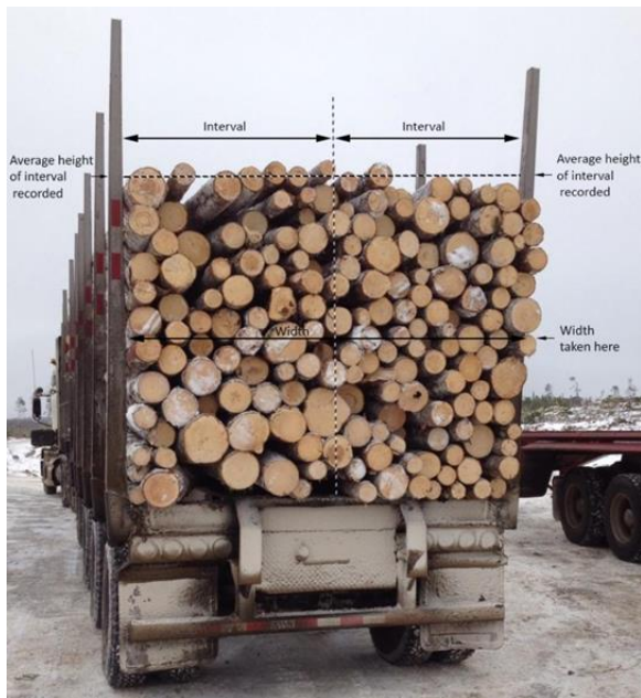
FIGURE 19 - RECORDING AVERAGE HEIGHT - WOOD STACKED EVENLY ACROSS THE TOP
