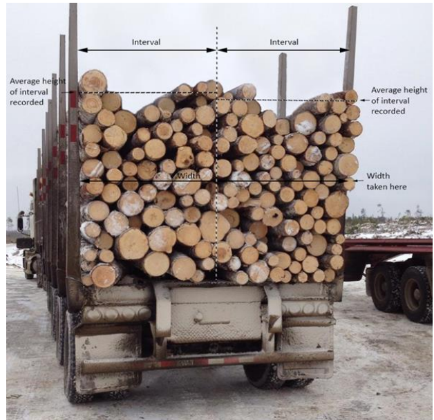
FIGURE 22 - RECORDING AVERAGE HEIGHT – WOOD STACKED IRREGULARLY
