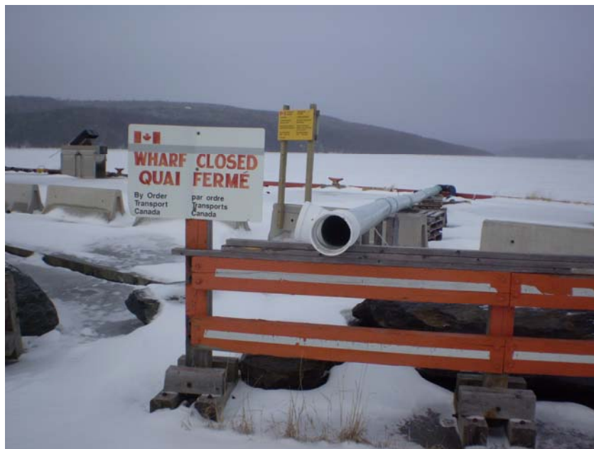
Photo 4.6.3.1 – Photo showing pipe shute extending across Transport Canada wharf for smolt delivery in spring and fall
