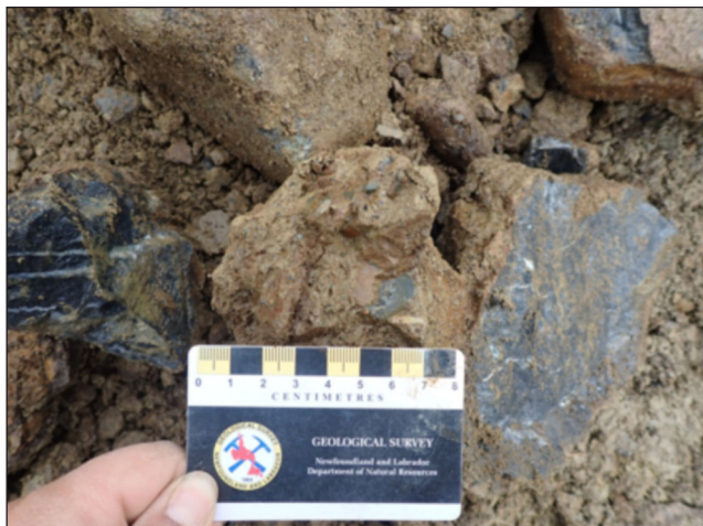
Plate 2. Compact sediment representing Till A sampled from 3 m at Site 5107. Appears lithified, clasts range from 0.2–20 cm.
