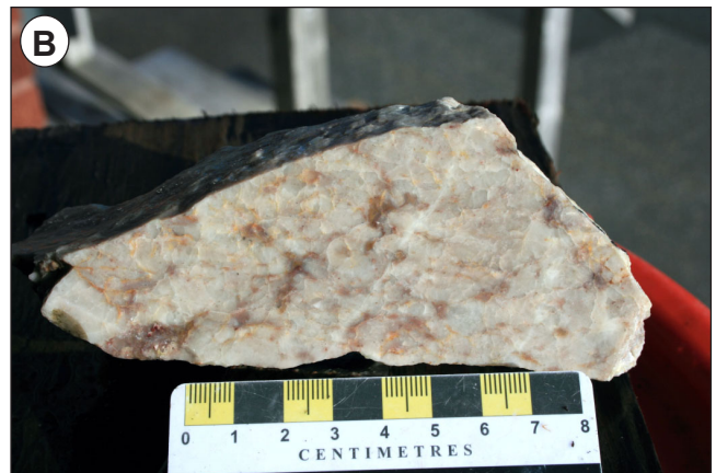
Plate 3. Photographs from the Tower alteration zone. A) Muscovite-dominated alteration in association with anomalous base-metal mineralization, 85 m depth; DDH BR-2K-08-005; B) Pyrophyllite–dickite alteration in an outcrop sample from the southeastern portion of the alteration zone.
