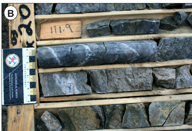
Plate 7. Photographs from the Woodman’s Brook alteration zone (DDH BE-95-003). A) Sharp transition from Fe–Mg chlorite–muscovite-altered felsic volcanic rock to a quartz-phyric, muscovitic illite-altered felsic unit (60 m depth). B) Base-metal-rich stockwork-style mineralization associated with muscovitic illite–muscovite alteration (112 m depth).
