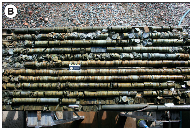
Plate 6. Photographs from the Seal Pond alteration zone (DDH SP-95-001). A) Gradational transition from Fe–Mg chlorite–phengite (top) to Fe–Mg chlorite–muscovite (bottom) alteration within crystal tuff (83 m depth); B) Interval of well-developed muscovite alteration locally associated with anomalous copper mineralization (100 m depth).
