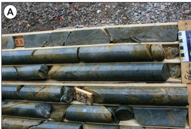
Plate 3. Photographs from the Tower alteration zone. A) Muscovite-dominated alteration in association with anomalous base-metal mineralization, 85 m depth; DDH BR-2K-08-005; B) Pyrophyllite–dickite alteration in an outcrop sample from the southeastern portion of the alteration zone.
