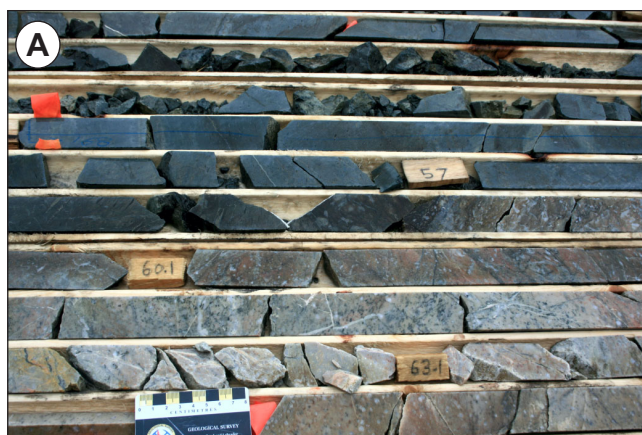
Plate 7. Photographs from the Woodman’s Brook alteration zone (DDH BE-95-003). A) Sharp transition from Fe–Mg chlorite–muscovite-altered felsic volcanic rock to a quartz-phyric, muscovitic illite-altered felsic unit (60 m depth). B) Base-metal-rich stockwork-style mineralization associated with muscovitic illite–muscovite alteration (112 m depth).
