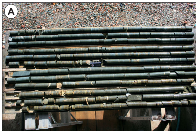
Plate 6. Photographs from the Seal Pond alteration zone (DDH SP-95-001). A) Gradational transition from Fe–Mg chlorite–phengite (top) to Fe–Mg chlorite–muscovite (bottom) alteration within crystal tuff (83 m depth); B) Interval of well-developed muscovite alteration locally associated with anomalous copper mineralization (100 m depth).
