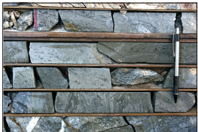
Plate 3. Massive sulphide mineralization locally assaying up to 36% Zn over 1 m; DDH 77537 at ~175 m depth (from Hinchey, 2011).
