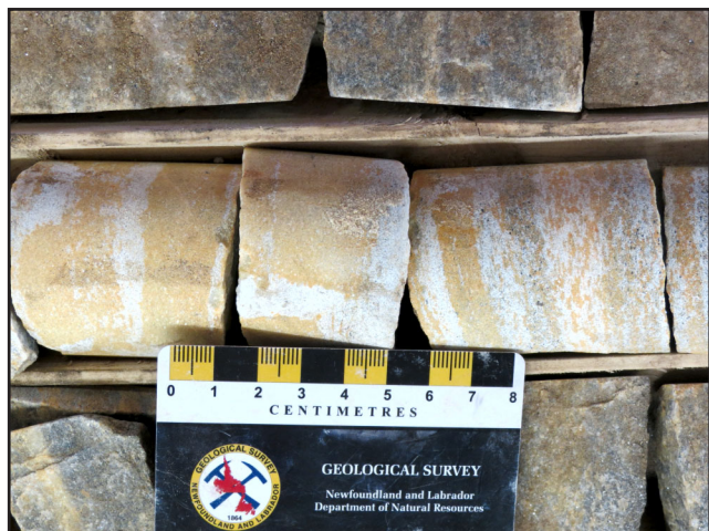
Plate 16. Carbonate-facies, with alternating bands of siderite–dolomite and quartz (from D’Aigle Bay 2 North prospect; drillhole DB-10-14 @ 165.9 m).
