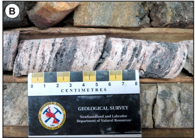
Plate 35. A) LIF close to the contact with Wishart Formation quartzite, with large euhedral garnets (drillhole J2-06-05 @ 117.3 m); B) Quartz–hematite oxide-facies iron formation (drillhole J2-06-05 @ 103.1 m).
