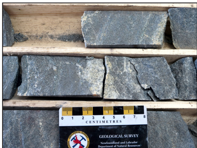
Plate 10. Mixed oxide-carbonate-facies iron formation with alternating bands of magnetite and carbonate-rich iron formation (from Wabush 3 deposit, drillhole W3-11-101 @ 212 m).
