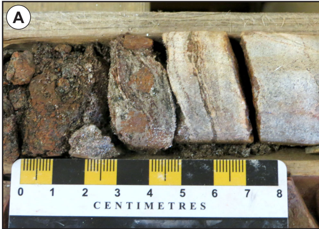
Plate 35. A) LIF close to the contact with Wishart Formation quartzite, with large euhedral garnets (drillhole J2-06-05 @ 117.3 m); B) Quartz–hematite oxide-facies iron formation (drillhole J2-06-05 @ 103.1 m).
