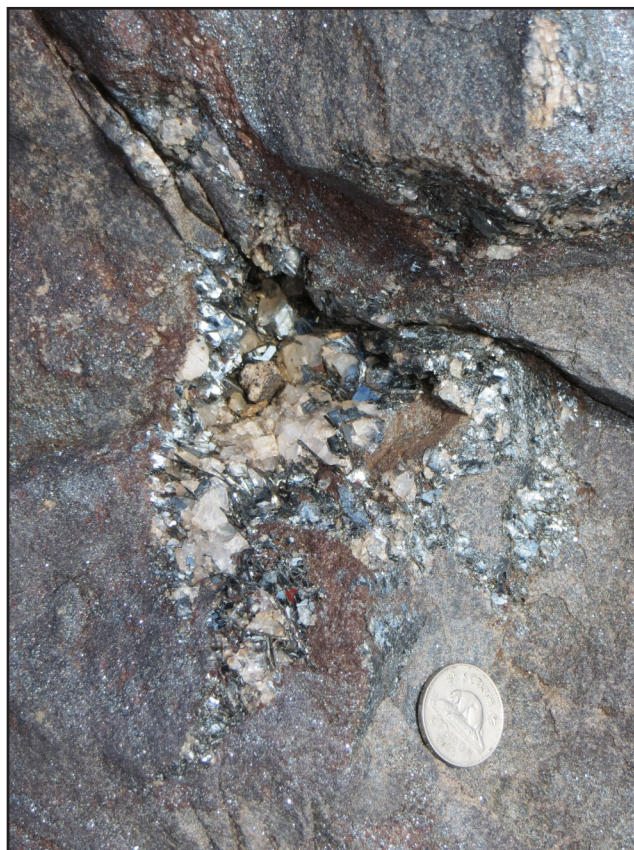
Plate 11. Oxide-facies iron formation, with coarse-grained specularite and quartz filling vug (from boulder in Carol Project).
