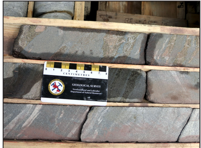
Plate 22. Mixed silicate and oxide (hematite) facies iron formation, with pink rhodochrosite (from Mills Lake deposit, drillhole K-10-95 @ 76.3 m).
