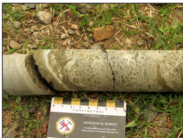
Plate 20. Garnet-bearing BSIF from the base of the Sokoman Formation in the Duley prospect (drillhole DU-10-03 @ 147 m).
