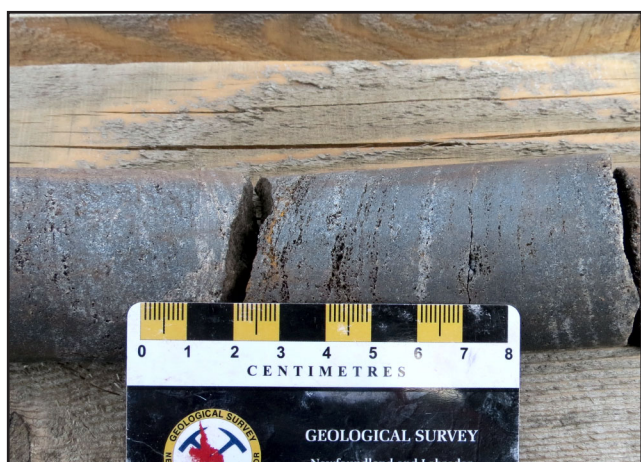
Plate 36. Quartz–hematite oxide-facies iron formation (drillhole J2-10-08 @ 153.2 m).
