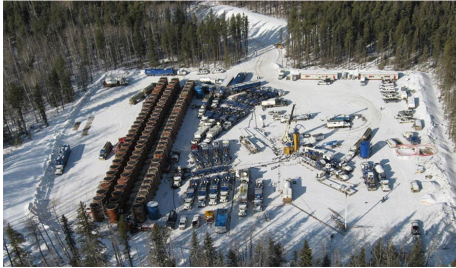
Figure 19. HF well stimulation in northwestern Alberta (courtesy of Trican Well Services).
