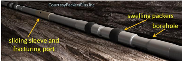
Figure 44. The ball drop and sliding sleeve method of completing a horizontal well.
