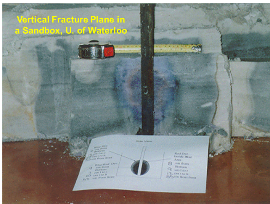
Figure 38. Vertical fractures develop when \sigma_{\text{hmin}} = \sigma_3 .
