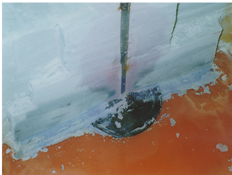
Figure 39. Horizontal fractures develop when \sigma_v = \sigma_3 .
