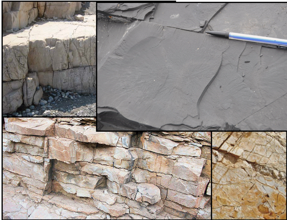
Figure 10. All naturally fractured low permeability rocks: but only one shale (upper rh photo).
