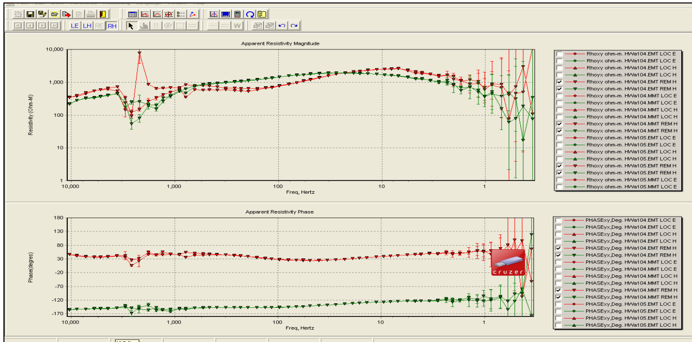
An image of MT data from MTEditor after data has been cleaned from the noise
