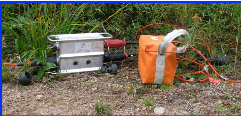
Aries RAM and battery - each RAM handles 8 channels A/D
