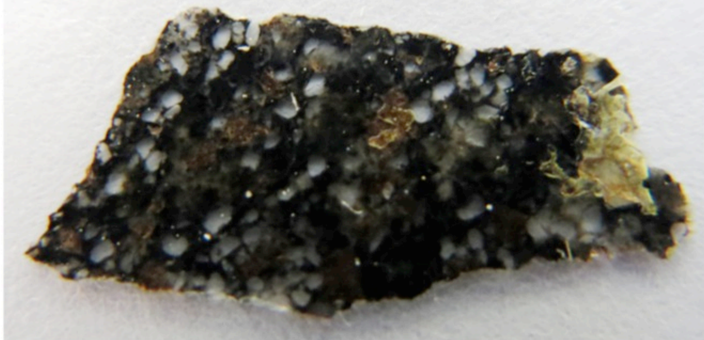
Figure 1. Sunday Run Formation sample showing quartz pebbles. This is a specially prepared fluid inclusion wafer. Pebbles are <5mm across and contain an abundance of fluid inclusions (FI) containing fluids that are at least 2 billion years old. These FI are the focus of this study.
