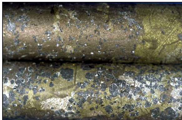
Ni—Cu—Co ore from the Voisey's Bay project, Vale Newfoundland and Labrador Limited
