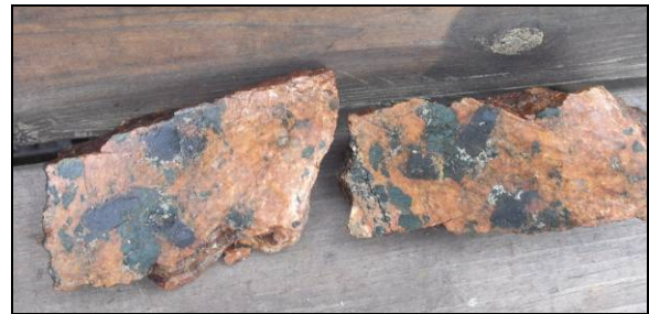
Coarse-grained allanite (black) and pyroxene (green) in granitic pegmatite from Silver Spruce's Pope's Hill Property
