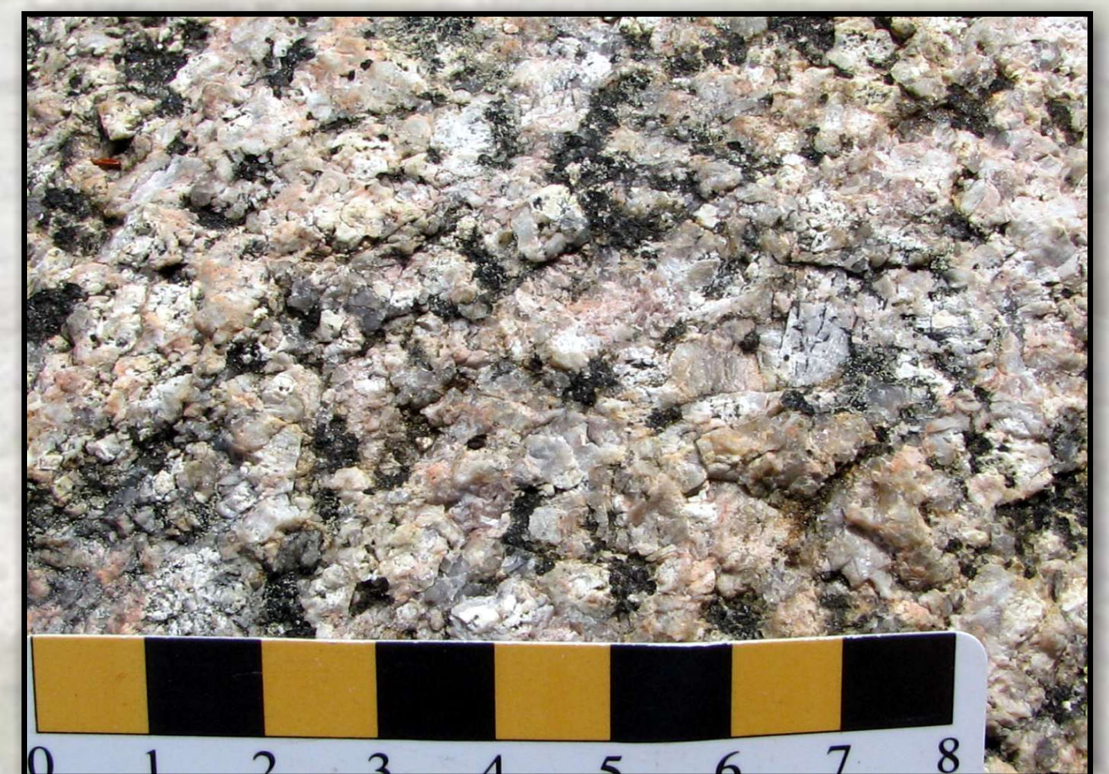
Coarse-grained, magnetite-biotite monzogranite from the Big River Granite (ca. 1800 Ma). The granite contains plagioclase phenocrysts (2 - 6 mm long) that are rimmed by K-feldspar.
