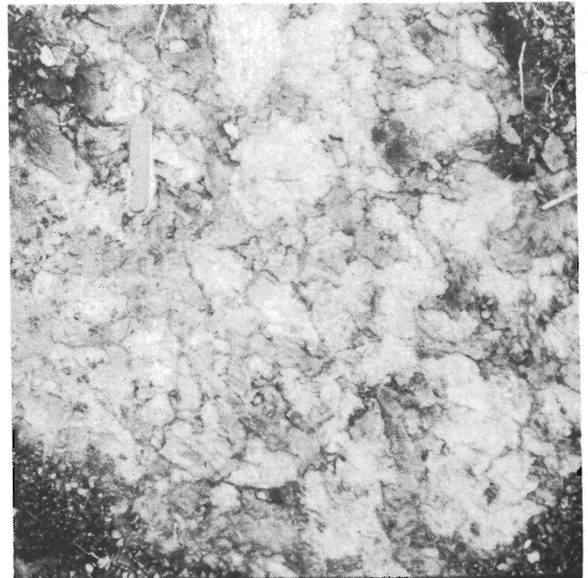
Plate 9: Very coarse grained isotropically textured norite (subunit 3g); plagioclase is mostly polygonized, some of the orthopyroxene is kinked. The penknife is 9 cm long. M&E-SW85-CS1-34.
