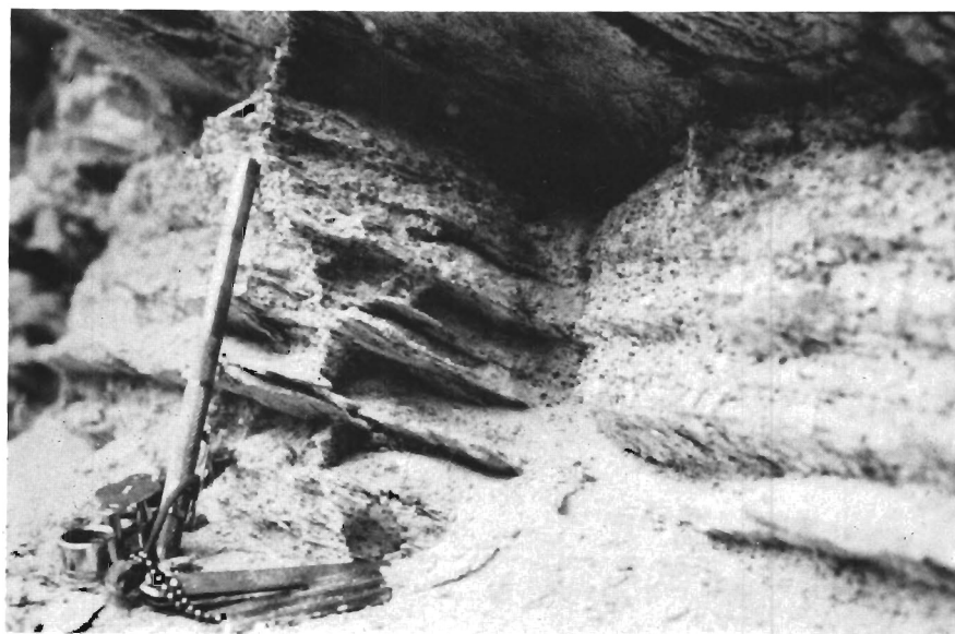
Plate 5: Clay-altered shale of the Simms Ridge Formation at the Browning prospect. Dark spots are siderite crystals.
