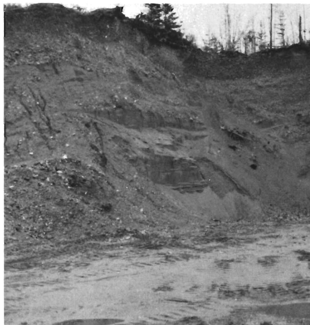
Plate 6. Fourteen-m-high quarry exposure showing stratified gravel and sand in Zone 22 .
