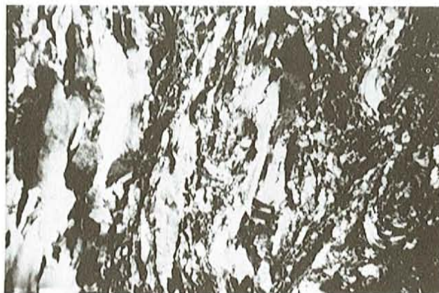
Plate 9. Strained quartz showing undulating extinction; field of view is 5 mm.
