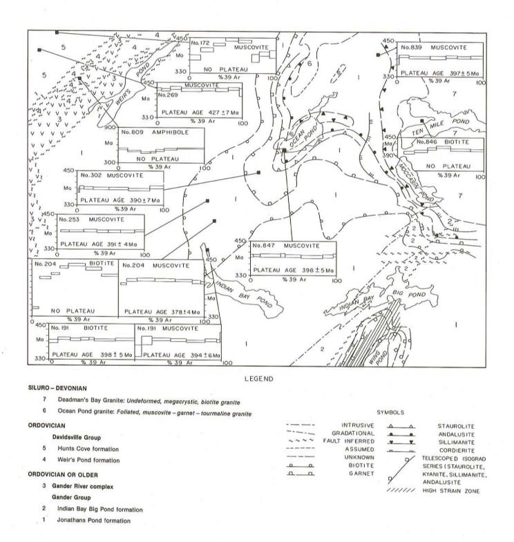
Figure 1. Geology and 40Ar/39Ar mineral age spectra for the Weir's Pond map area, northeastern Gander Zone, Newfoundland.
