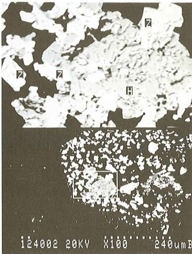
Plate 2. SEM backscatter photograph of euhedral zircon (Z) intergrown with hematite (H); black is silicate gangue; scale bar refers to lower half of photo; scale of top (area in box) is 5x scale of bottom; sample JT-124.
