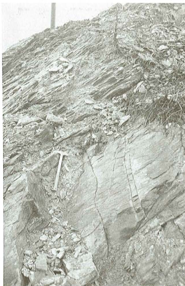
Plate 3. Highly deformed quartz—sericite \pm fuchsite—pyrite schist associated with shear-hosted ore; footwall of Main ( Rambler) orebody.
