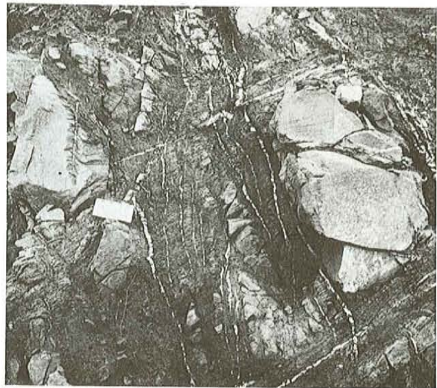
Plate 2. Blocky alteration and quartz veining (Trench 12). Shearing, alteration and quartz veining follow jointing developed within the gabbro; blocks are remnants of less altered gabbro.
