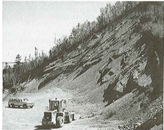
Plate 8. Sandy gravel, gravel and cobble-gravel visible along 20-m-high quarry exposure in the Browns Arm delta deposit.
