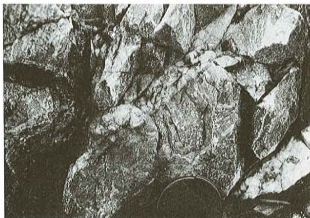
Plate 1. Brittle-controlled auriferous quartz vein (78.2 g/t Au) developed in siliceous felsic dyke, Powderhouse Cove.
