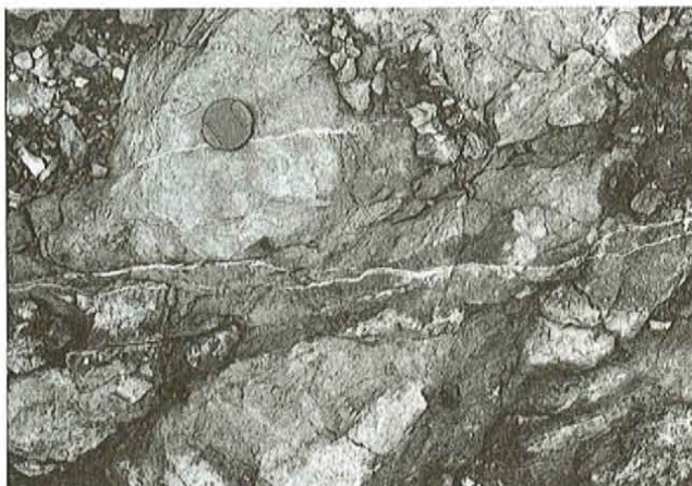
Plate 3. Shear-zone-controlled quartz veins with intense hematite alteration haloes developed within altered ultramafic rocks, Breccia Pond.
