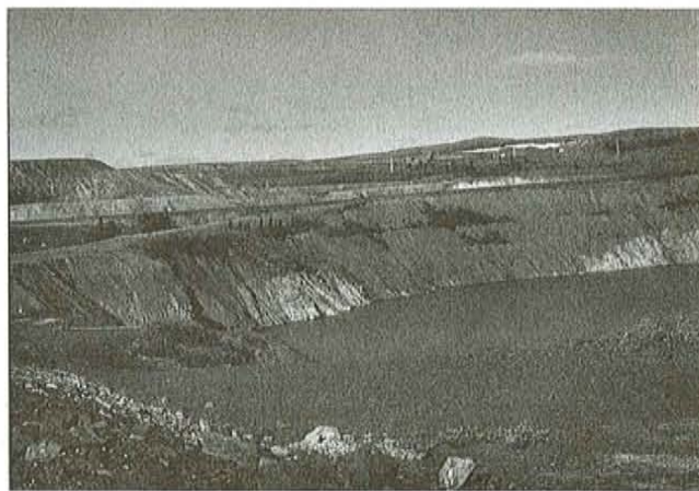
Plate 4. West wall of Burnt Creek mine, showing up to 30 m of surficial sediment exposed in broad bedrock low.
