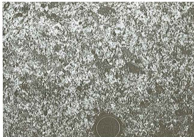
Plate 13. Weakly foliated to massive K-feldspar megacrystic monzonite (Unit 4mp). K-feldspars locally have recrystallized rims; Mealy Mountains terrane.
