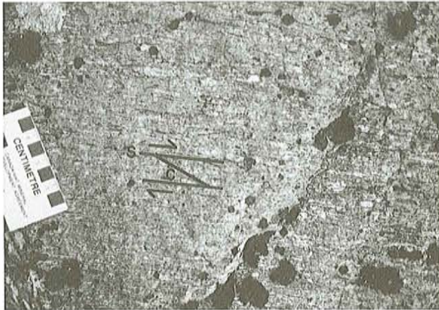
Plate 1. Mylonitic granite showing C-S fabric suggesting dextral (west over east movement); enclave in gabbro of White Bear Arm complex. S-foliations; C-shear band.
