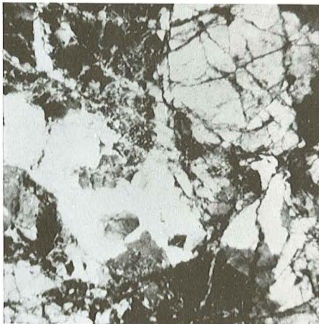
Plate 6. Microfractures in quartz and feldspars crystals.
