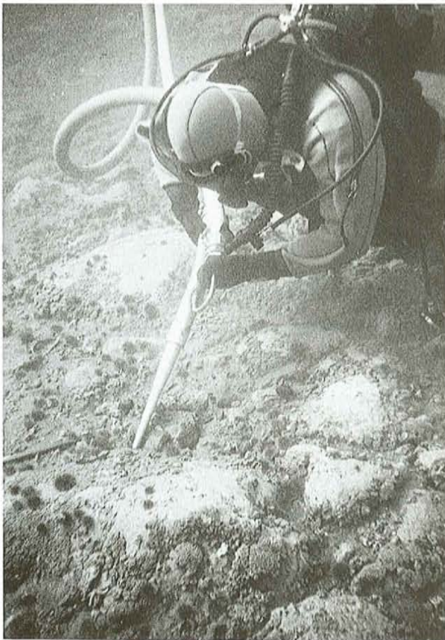
Plate 2. Diver-operated suction sampler.
