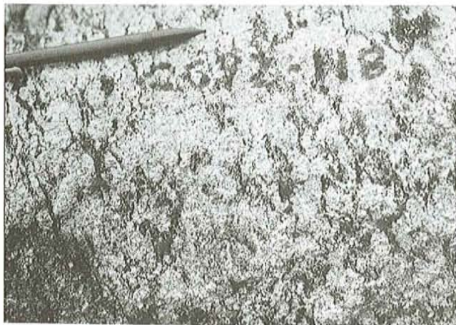
Plate 2. Anorthosite from the western part of the map region. A partially retrograded garnet is present in the lower central part of the photograph.
