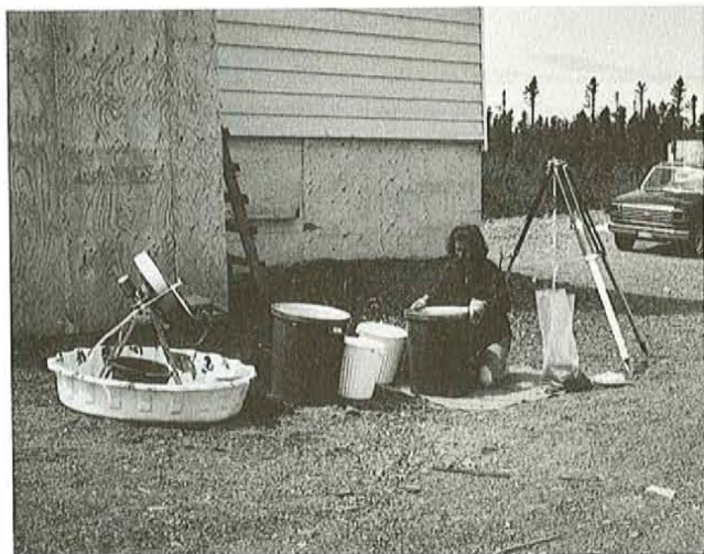
Plate 1. Methodology for processing a sample. A combination of sieving and Goldhounding.
