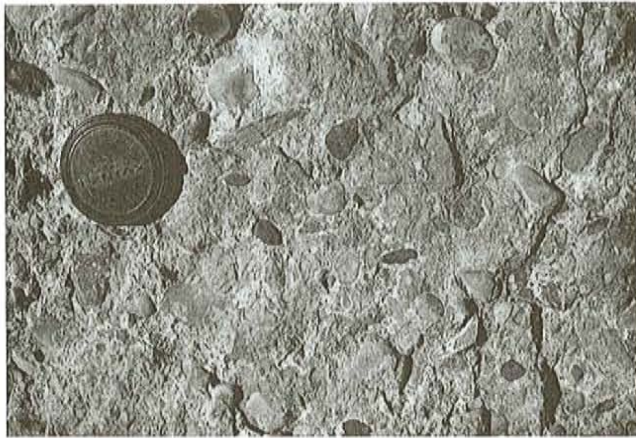
Plate 1. Sandstone showing reactive rims around the pebbles.
