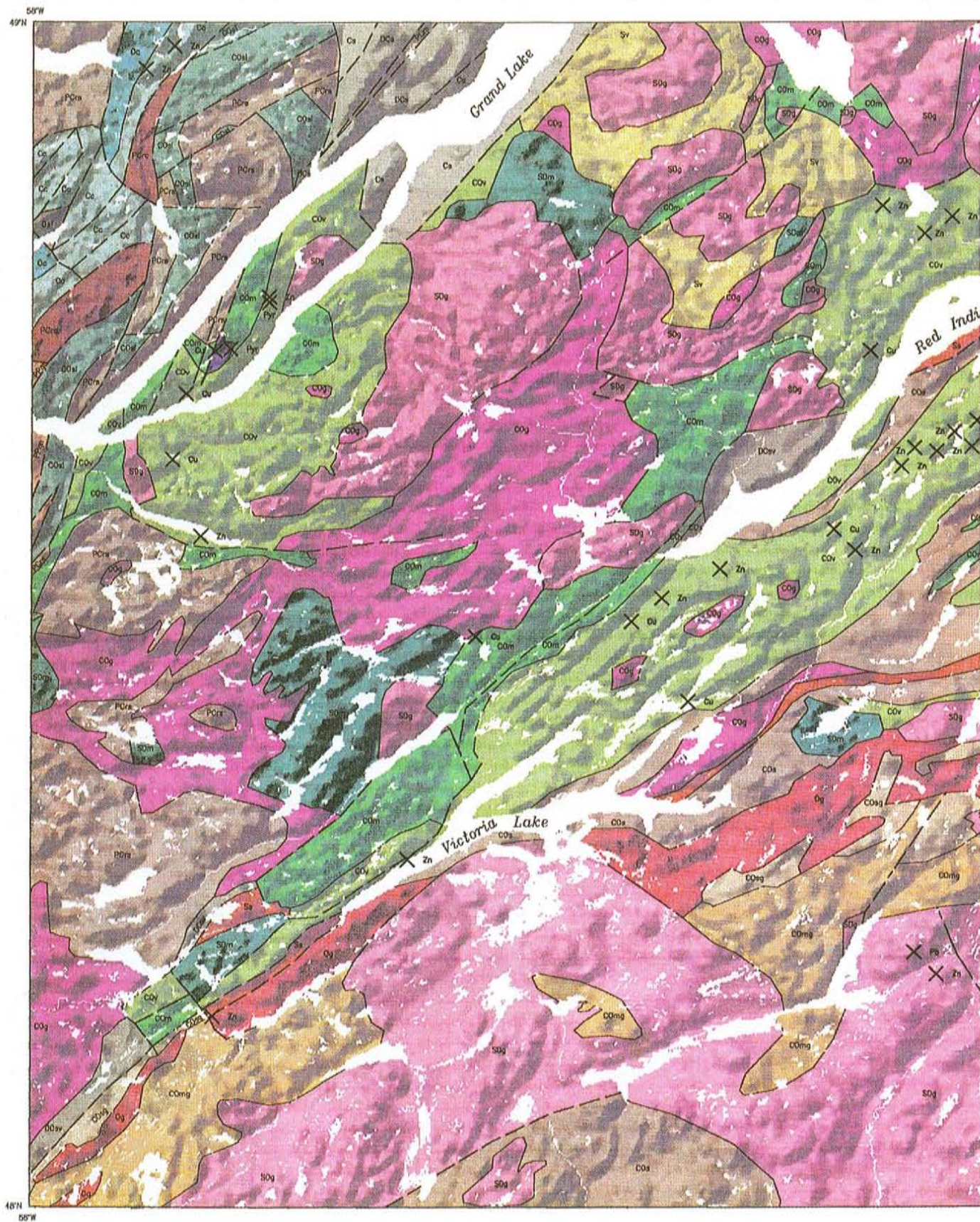
Figure 3. Geology draped over digital terrain model of the Red Indian Lake map sheet, NTS 12A; false illumination from the northwest. Figure also shows massive sulphide occurrences and bedrock geology draped on shaded topographic surface.
